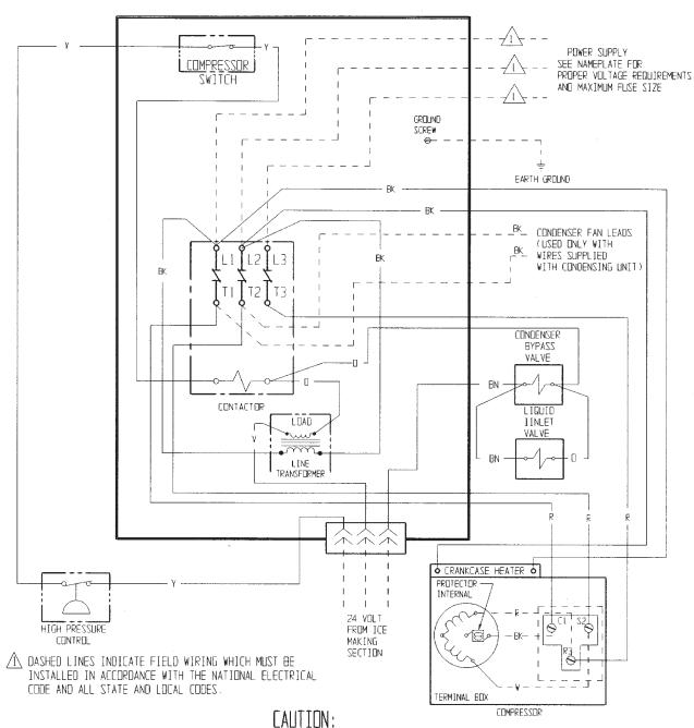
THIS UNIT MUST BE GROUNDED. MORE THAN ONE DISCONNECT MEANS MAY BE REQUIRED TO DISCONNECT ALL POWER TO THIS UNIT.
