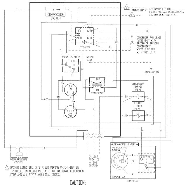
THIS UNIT MUST BE GROUNDED. MORE THAN ONE DISCONNECT MEANS MAY BE REQUIRED TO DISCONNECT ALL POWER TO THIS UNIT.
