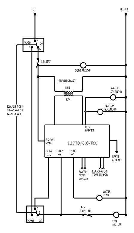
SWITCHES ON THIS UNIT SHOWN IN FREEZE CYCLE
