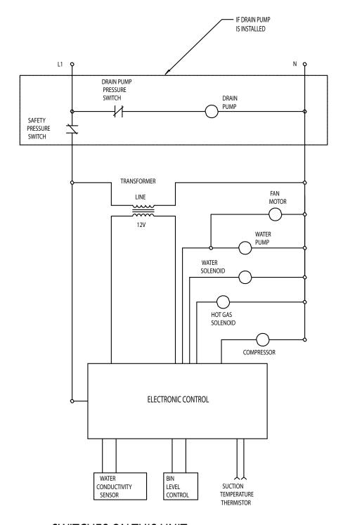
SWITCHES ON THIS UNIT SHOWN IN FREEZE CYCLE WITH DRAIN PUMP IN OPERATION AND BIN DOOR CLOSED
