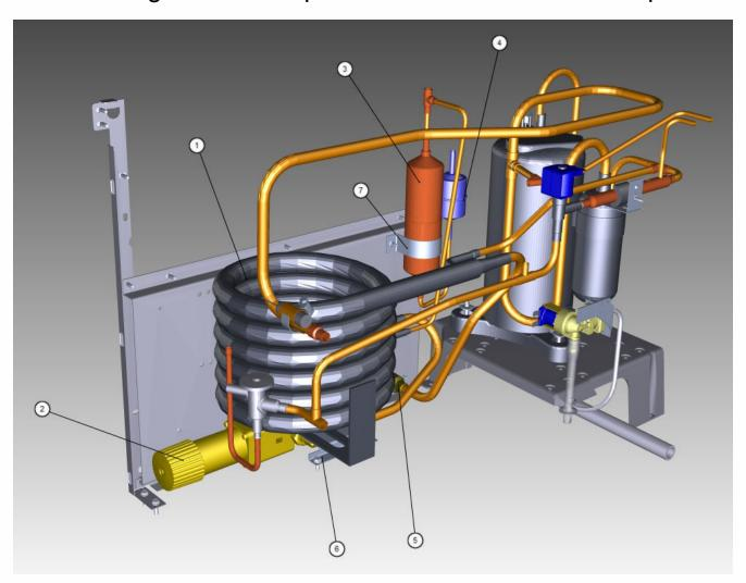
K0500 Refrigeration Compartment - Water-cooled Components
