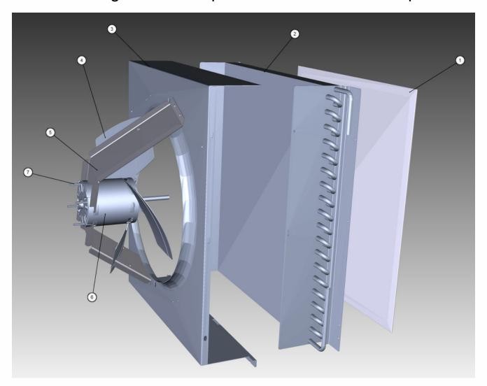
K0500 Refrigeration Compartment - Air-cooled Components
